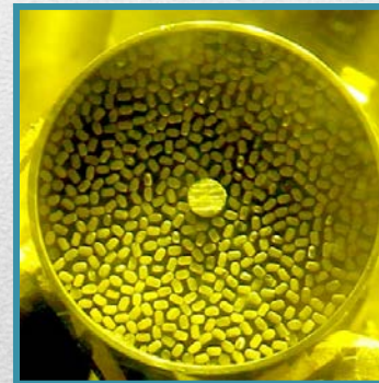
▲ Cutting of IVG.1M HEU-Fuel after Reactor Tests
